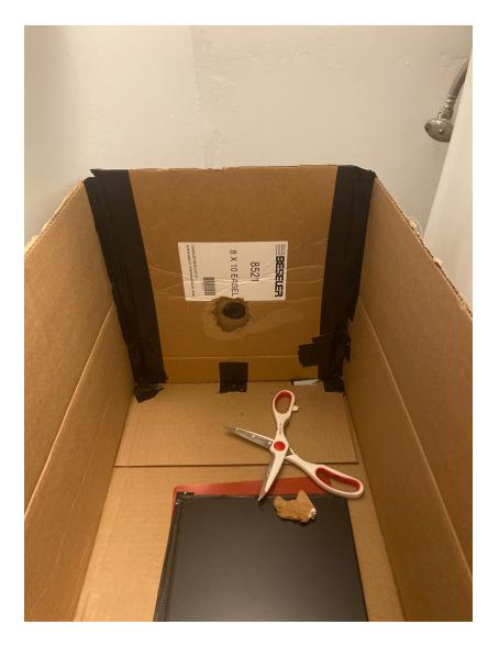
Cardboard enlarger from the bottom view up, the hole is where the magnifying glass is. The red sheet was slid into a little space made at the top to make the LED light less harsh.
