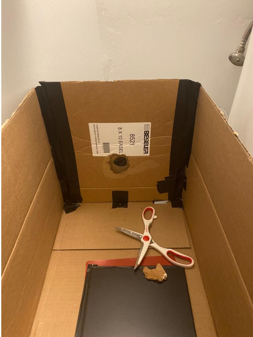
Cardboard enlarger from the bottom view up, the hole is where the magnifying glass is. The red sheet was slid into a little space made at the top to make the LED light less harsh.
