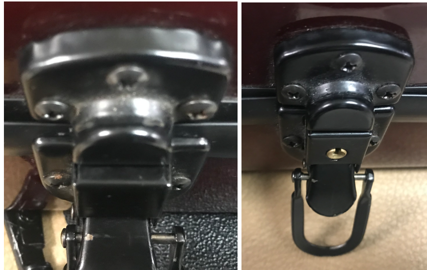
Figure II. The clip in the image on the left is unaligned between the top and bottom, which is causing there to be a lip on the bottom of the clip and resulting in the case not closing the entire way. The clip on the right is properly aligned so that the top and bottom of the clip align.
